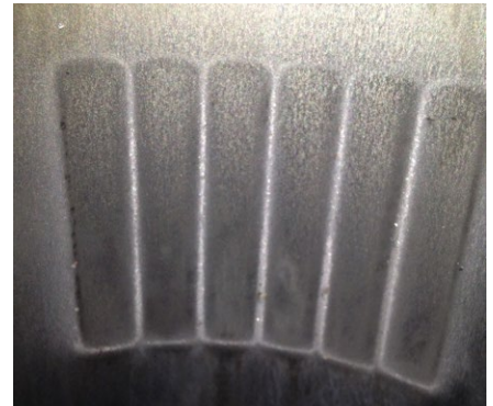
Stage 2: Normal wear will show a light dusting of captured particles.
