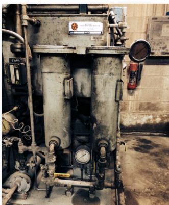
The SAG Mill's two 16" diameter canister filters.
