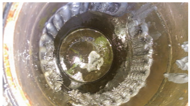
Millions of microscopic particles captured by FilterMag in only 70 hours of crusher operations. Most are small enough to pass through the filter.
