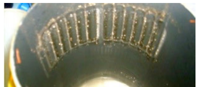
Nibral particles captured by FilterMag in each of the four high pressure filters.
